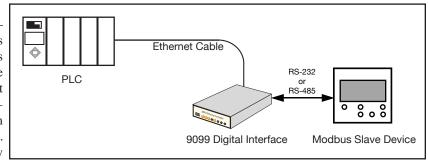
Using a 9099 as a Modbus TCP/IP to Modbus RTU Converter
