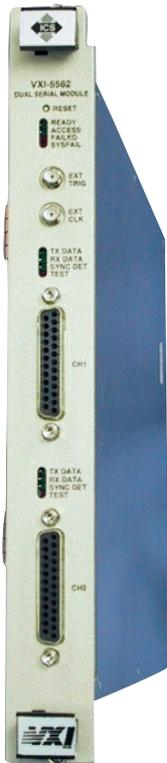
PLEASANTON, CA, July 26, 2002. Today ICS Electronics announced a new dual channel VXI to Serial Interface Module. This new VXI module provides two high-speed serial channels for transmitting and receiving binary data. The Model VXI-5562 is a register based module with large FIFOs and other features to support continuous high-speed data transmission. Applications include testing devices with binary data patterns and Satellite Command and Telemetry systems.
