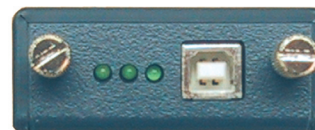
488-USB rear view showing USB connector and diagnostic LEDs
