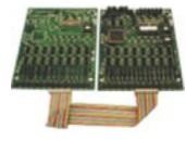
PLEASANTON, CA, January 29, 2007. Today, ICS Electronics announced a new GPIB-to-Parallel Interface for interfacing devices with TTL, CMOS or other digital signals to the GPIB bus. Designated the Model 4813H, this two board set expands the number of digital I/O lines available in OEM boards up to 256 lines. Typical applications for the 4813H are interfacing test
