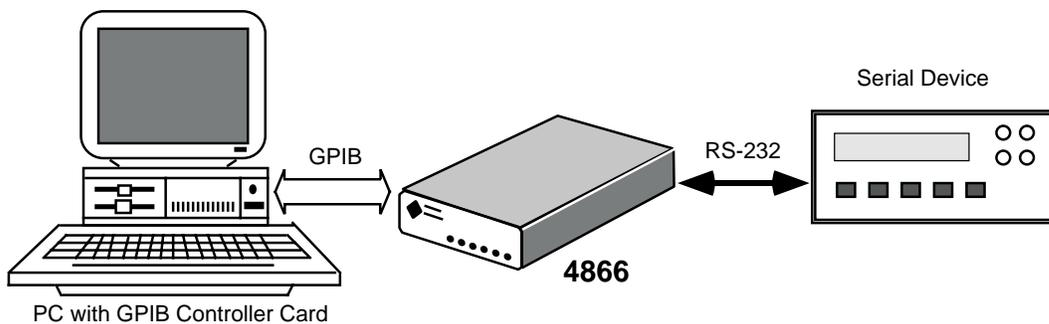
Figure 2(b) 4866 with a Standard Serial Device
