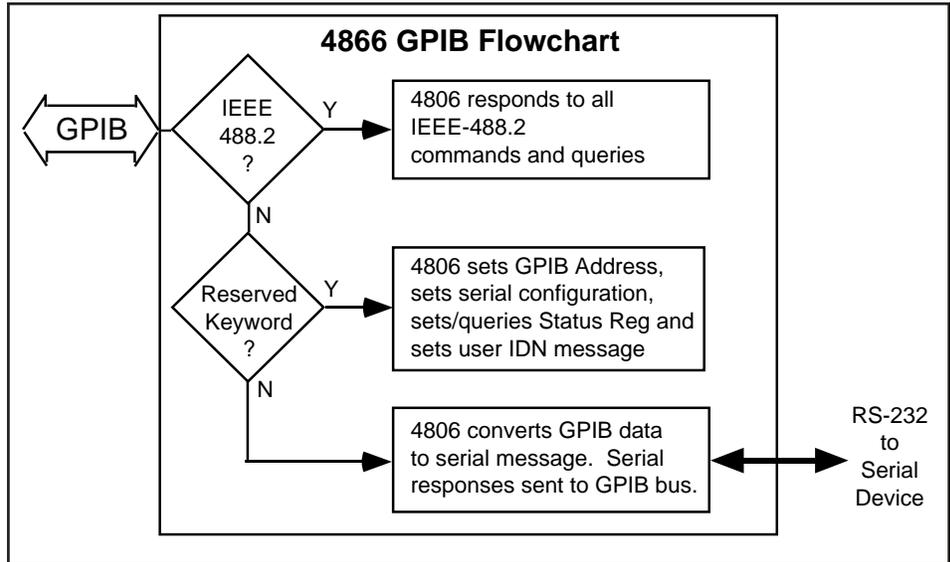
Figure 3 4866 Operation Diagram
