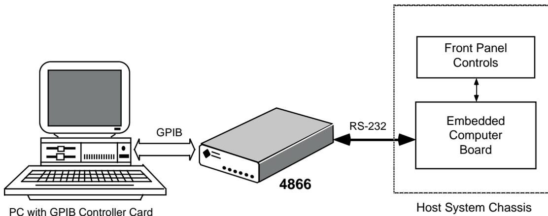
Figure 2(c) 4866 with a Smart Serial Device
