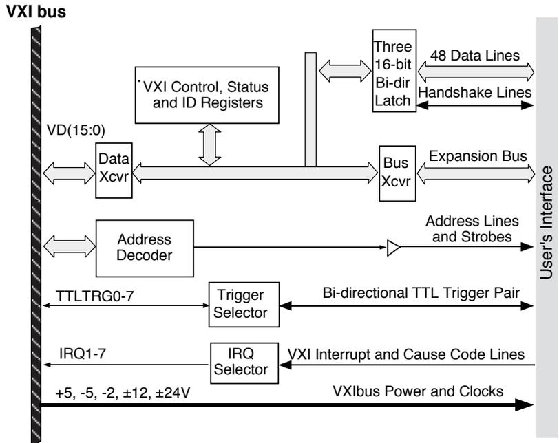
Figure 1 VXI-5524A Block Diagram
