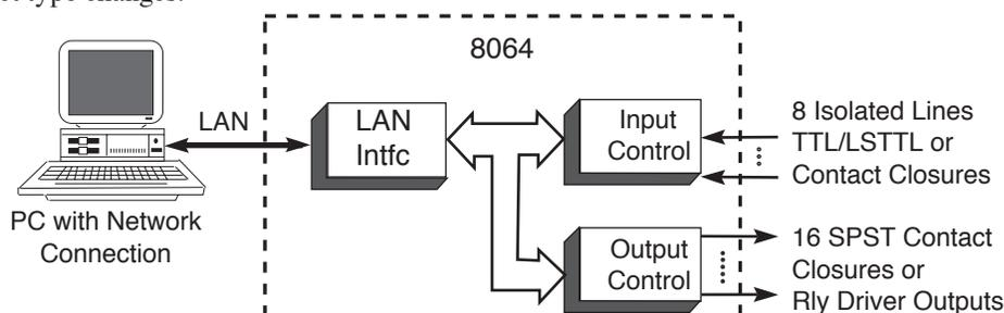
Figure 1 8064 Block Diagram
