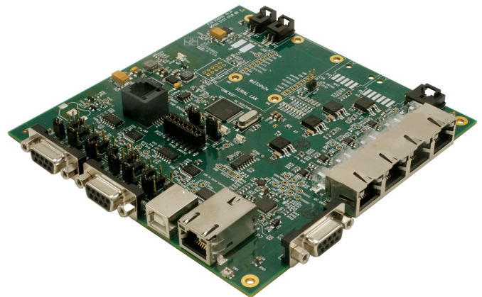
MSC02 System Controller Board with Ethernet, USB and Serial interfaces.
