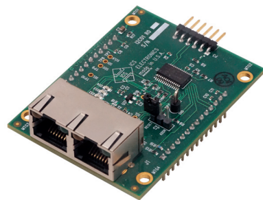
Small I2C01 Switch Module showing the dual I 2 C bus connectors
