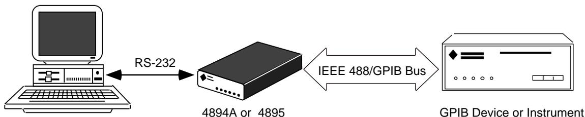
Figure 1 Serially controlling a GPIB Device
